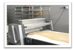
A worker at a Winnipeg Bakery amputated three fingers with a moving scraper blade when attempting to clean a piece of equipment used to cut dough. The employer was prosecuted and fined \$43,800 for failing to ensure that a worker did not clean a dough dividing machine without the
